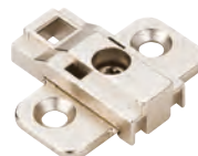
400.0P74.05 ZINC DIE CAST, NICKEL PLATED ■ PREASSEMBLED WITH 6.3MM X 15MM EURO SYSTEM SCREWS ■ HEIGHT ADJUSTMENT: +/- 2MM
