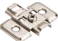
400.0P73.05 COLD ROLLED STEEL, NICKEL PLATED ■ PREASSEMBLED WITH 6.3MM X 15MM EURO SYSTEM SCREWS ■ HEIGHT ADJUSTMENT: +/- 2MM
