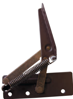
CH5-BR BROWN POWDER FINISH ■ SPRING LOAD ■ LID SUPPORT OVER CENTER STAY OPEN, SOFT CLOSE BEYOND CENTER
